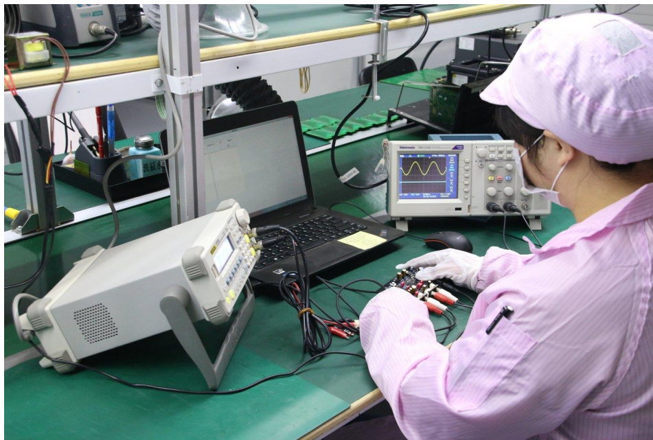
Figure 29 - Bittele Test Engineer Performing FCT on an Assembled Board
