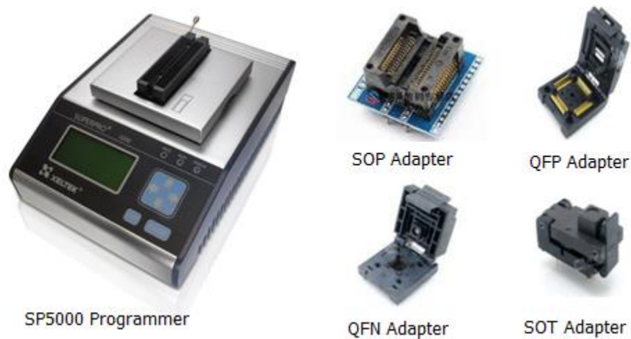
Figure 22 – Some of Bittele's Direct-Chip Programming Equipment
